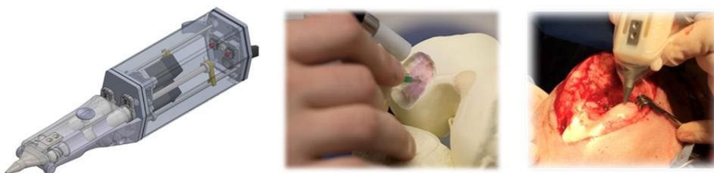
Figure 1: The Biopen is a handheld device for surgical bioprinting.
